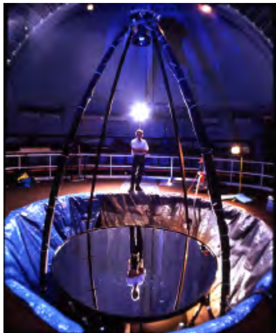
Graduate student Mark Mulrooney in the Liquid Mirror Telescope he has helped design, test, and build (photo courtesy Chip Simons).
