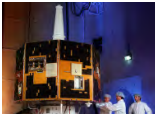
The IMAGE spacecraft getting readied for launch in February 2000 depends on neutral atom imaging to view particles trapped in Earth's magnetic field.
